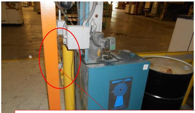
System is disabled. It was mentioned that this is a legacy Lubrication system and parts are no longer available. This System has a broken circuit board that has been out for Repair for the last 8 weeks. Lack of lubrication is a <u>MAJOR</u> issue on this type of conveyor system.
